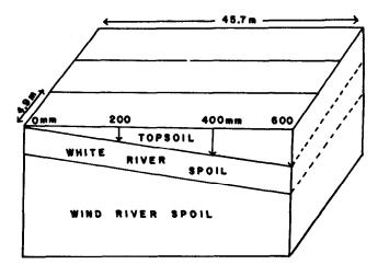
Fig. 1. Diagram of reconstructed soil with variable topsoil depths.
